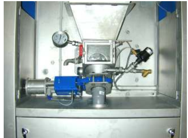
Mixing box with draining and steam connection
