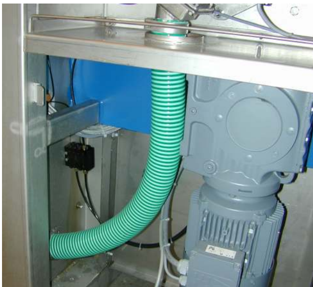
VG drive, draining pipe and central lubrication
