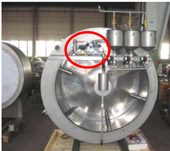
Water mixing and dosing system
